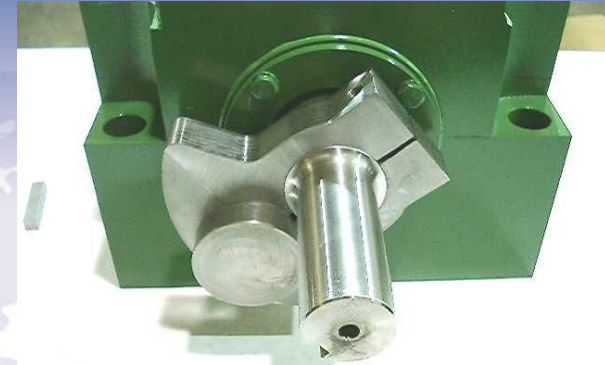
STEP 2 Install counter weight
