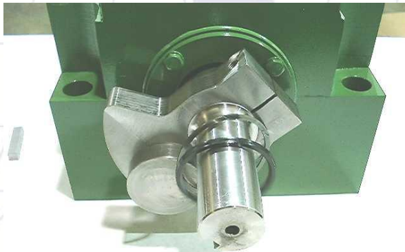
STEP 3 Install snap ring and seal
