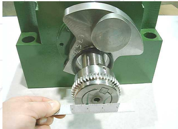
STEP 7 Install hub so it is flush with end of shaft
