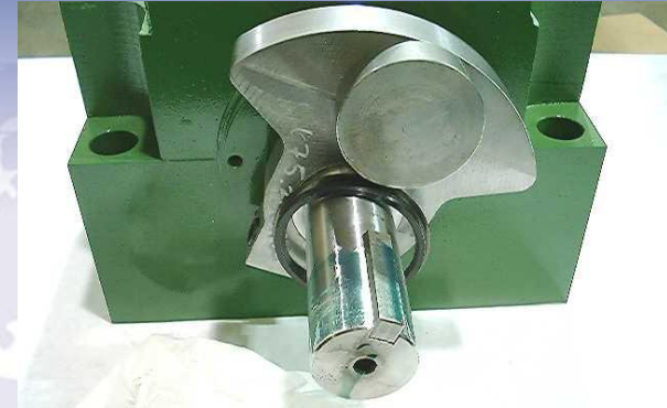
STEP 6 Apply 603 loctite to shaft and key
