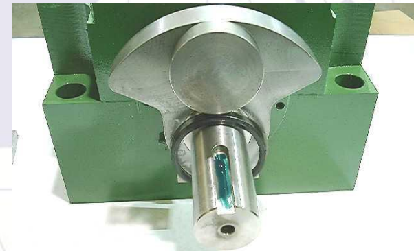
STEP 4 Use 603 loctite in key-way
